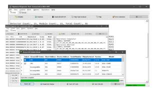
Now with v1.8, programmers can use this software and the HDT to select the LED inhibit feature of Signature Optica detectors. This allows for turning off normal green polling led applications that require no background flashing in non emergency conditions. (Requires detectors with 1.0.16 or later firmware.)
